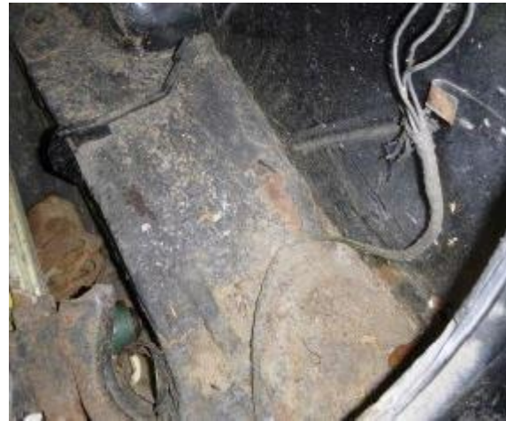
Boot - bituminous layer which contained chrysotile asbestos
