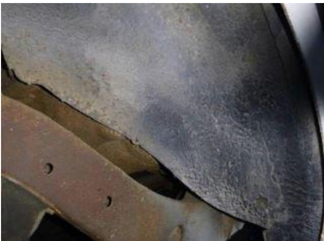
Underbody bituminous layer which contained chrysotile asbestos
