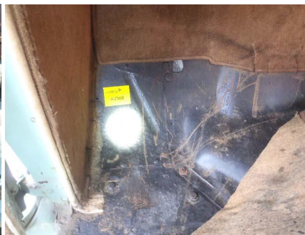
Mastic on floor pan which contained chrysotile asbestos
