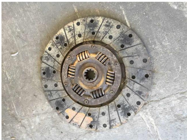
Clutch plate which contained chrysotile asbestos
