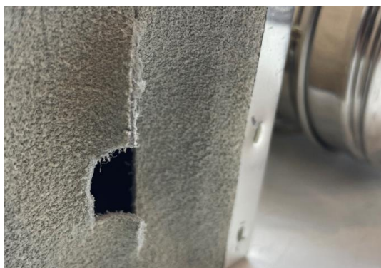
Bellows material cut for analysis
