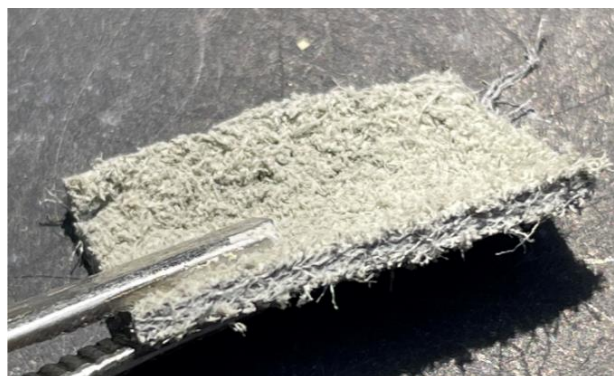
Material with visible asbestos fibres
