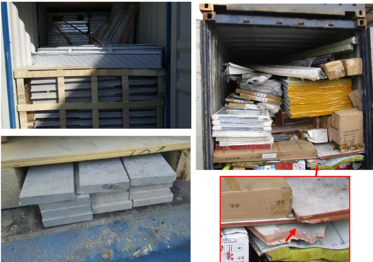
Figure one shows chrysotile asbestos detected in cement fibre boards and two shows chrysotile asbestos detected in cement fibre boards, shipped as part of a prefabricated house kit (source: ABF, https://www.abf.gov.au/prohibited-goods-subsite/files/ABF_detections_of_asbestos.pdf )
