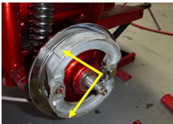
Figure 1: Brakes on motor scooter side-car which contained asbestos
