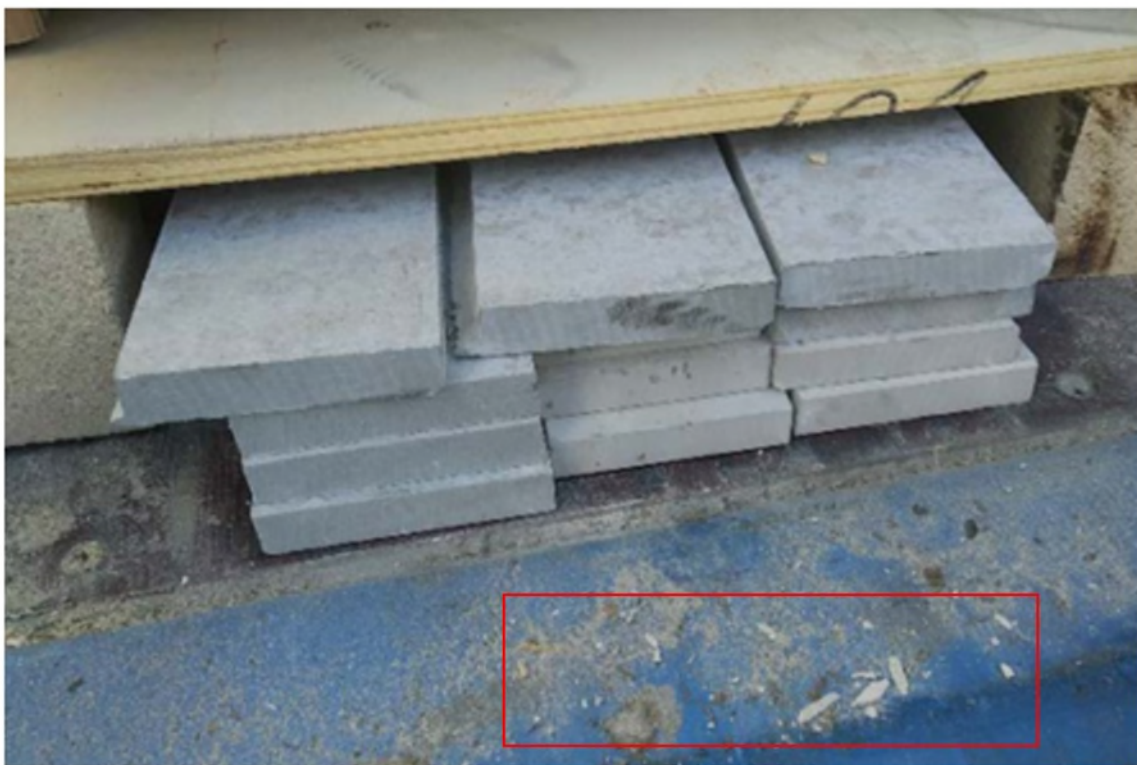
Debris from the boards was present on the container floor.
