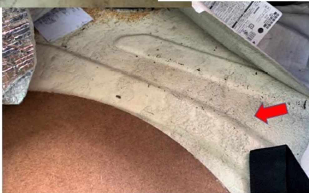
Bituminous mastic painted onto interior of boot
